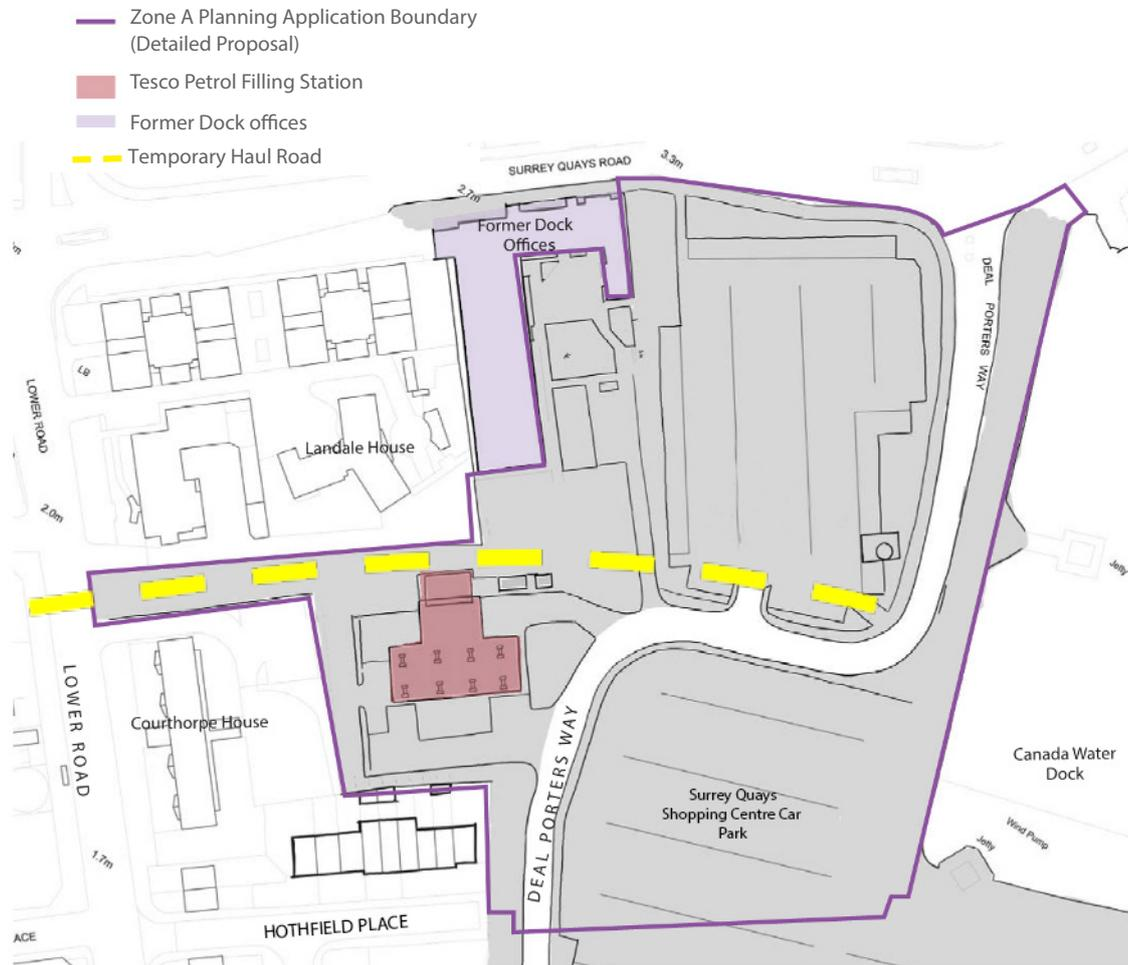
Figure 1: Mark-up showing the alignment of the temporary haul road
